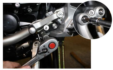
7 Stack the side stand mount casting on top of bar and then begin threading the (a) (2) OEM M10 side stand bolts back into place. Do not tighten all of the way. Next tighten the (b) (2) T45 peg mount bolts. Now you can tighten the (4) M8 crash bar fasteners to 18nm of torque and then the (2) M10 side stand bolts to 70nm of torque.
