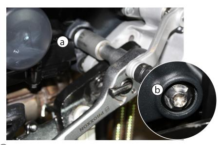
On the riders left side, re-install the engine bolt (a) nut using a 17mm socket. Tighten this to 105 nm of torque. You may need to use the supplied T55 driver to keep the (b) bolt from spinning.
