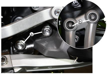
With bike on center stand, remove the (a) (2) M10 kick stand bolts using a 12mm socket. Loosen the (b) (2) T40 foot peg bracket bolts halfway, this provides access to next nut. When this assembly is loose be cautious of the vulnerable side stand switch.
