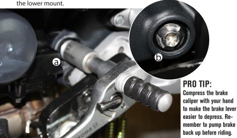
3 Using a 17 mm socket, remove the (a) nut from the 12 mm engine bolt. You may need to hold the (b) bolt head end with the provided T55 driver. With nut removed slide the bolt out of the engine. You can drive the bolt out with a 1/4" extension if there is resistance.
