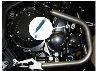
(4) Install the right side crash bar by starting with the (a)M8 x 30 mm fastener and washer to the radiator mount and following with the (b)M8 x 25 mm fastener and washer using thread locker. Complete right side by re-installing the 12 mm engine bolt. Do not completely tighten any fasteners just yet. Use 1/4" driver to push the 12 mm engine bolt if needed.
