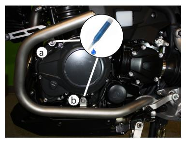
(6) With the side stand still removed, install the left side bar. Start with the (a)M8 x 30 mm bolt and washer that attaches to radiator mount. Next install the (b)M8 x 25 mm lower mount bolt with washer and thread locker for both bolts. Do not tighten either bolt completely.
